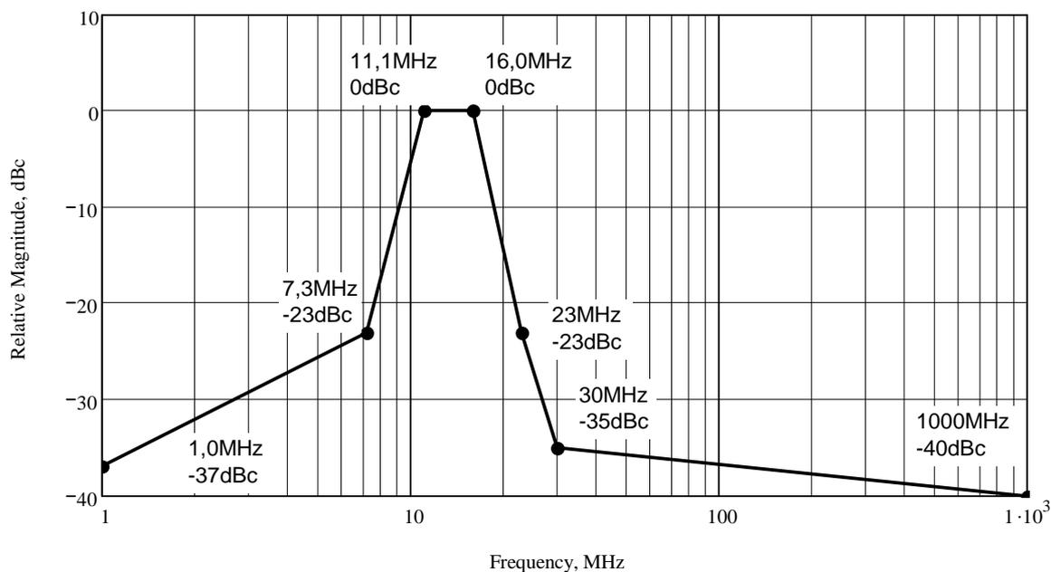
**Figure 2: Euroloop transmitter spectrum and spurious mask**
